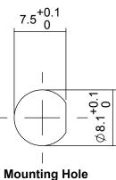
Dimensions in mm (typical) Not to scale Anode termination denoted by red indicator Mounting hole to be clean and burr free
